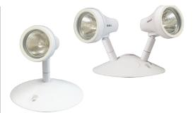
The S series of commercial MR16 remotes provides exceptional light output in a compact, traditional design. The die cast, all metal housing is fully adjustable with a friction lock tilt and swivel that can be locked in place with a rear mounted set screw. The canopy is designed to mount directly to typical electrical junction boxes. Available in 6 V, 12 V and 24 V models, all utilizing low glare LED lamps.
