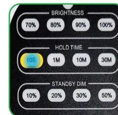
Select the desired HOLD TIME value for the luminaire by pressing the HOLD TIME button multiple times until the desired HOLD TIME value lights up in the DISPLAY AREA (10s / 1min / 10min / 30min).
