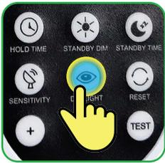
Long press (3-5 seconds) the "DAYLIGHT" button until the "DAYLIGHT" indicator light is ON in DISPLAY AREA (6 th row).
