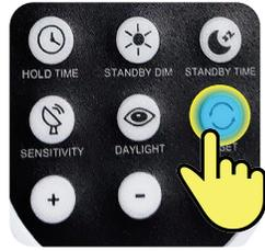
**TEST** The TEST button can be used to confirm that the sensor is functional. Pressing this button, the sensor goes to test mode (hold time is only 3s). Press again the button to quit from this mode.
