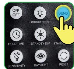
Press SEND button to save this setting. The luminaire will flicker once to confirm that the new setting is registered.
