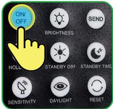
Press and hold for 3-5 seconds the ON/OFF button until the BRIGHTNESS indicator light is on in DISPLAY AREA (first row).
