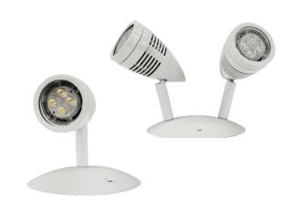
The RMMB series of commercial MR16 remotes provides exceptional light output in a compact, traditional design. The die cast, all metal housing is fully adjustable with a friction lock tilt and swivel that can be locked in place with a rear mounted set screw. The canopy is designed to mount directly to typical electrical junction boxes. Available in 6 V, 12 V and 24 V models, all utilizing low glare, MR16 LED lamps.
