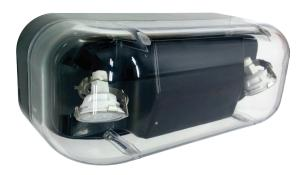
The EBN series of battery units is designed to operate in the most extreme environments. The unit, designed using a polycarbonate housing, maintains its sealed interior with a continuous integral gasket. The EBN series is available in 6 V DC and 12 V DC versions in 36 W, 50 W, 72 W, 100 W or 130 W wattage capacity for a minimum of 30 minutes in emergency mode. Auto test feature is standard.
