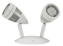
The RMMB series of commercial MR16 remotes provides exceptional light output in a compact, traditional design. The die cast, all metal housing is fully adjustable with a friction lock tilt and swivel that can be locked in place with a rear mounted set screw. The canopy is designed to mount directly to typical electrical junction boxes
