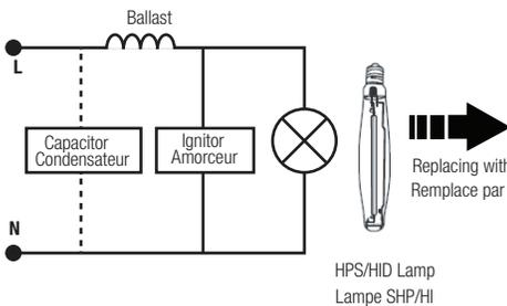
**LED RETROFIT LAMP WIRING DIAGRAM
