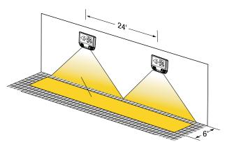
24' spacing on a 6' path mounted at 8'.
